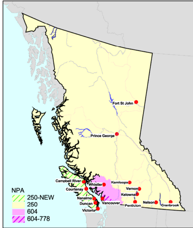
Figure 12 - Plan 3a - Concentrated Overlay on NPA 250 Vancouver Island area, and NPA 250 Mainland area grows with NPA 250
